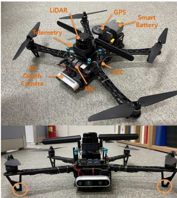
Fig. 3 Research drone installed with collision-avoidance system
