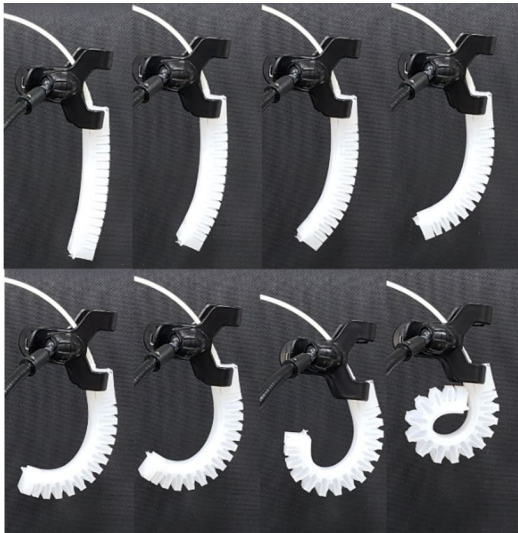
[Fig. 7] Bending angle of conventional PneuNets actuators: The actuator was captured between 0 to 17.5 kPa in 2.5 kPa increments
