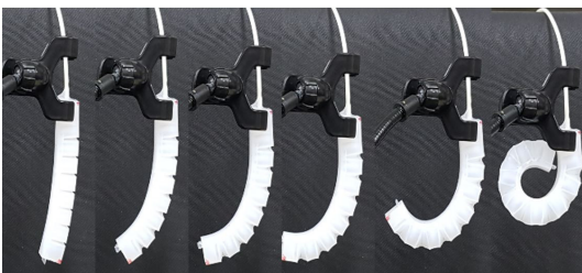
[Fig. 8] Bending angle of improved PneuNets actuators: The actuator was captured between 0 to 12.5 kPa in 2.5 kPa increments
