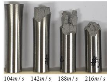
Fig. 7 Main parts of specimen after Taylor impact test
