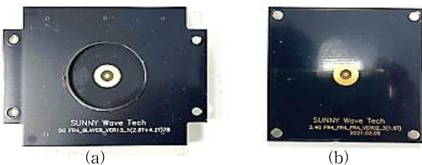
Fig. 6 Surface wave generator for ship's environment(a) and land use(b)
