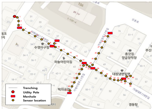
Fig. 1. Sensor location for Busan Yeon-je district
