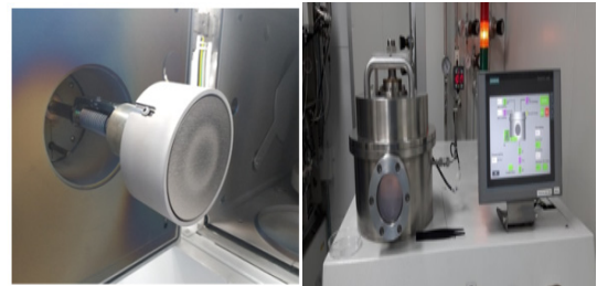
Fig. 6. Plasma treatment of a silicon substrate by surface oxidation method.
