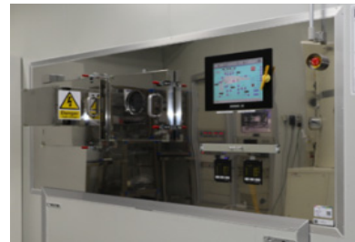
Fig. 7. DLC(Diamond-like-carbon) Coating Machine
