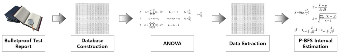
Fig. 1. The entire process of evaluation for performance of body armor
