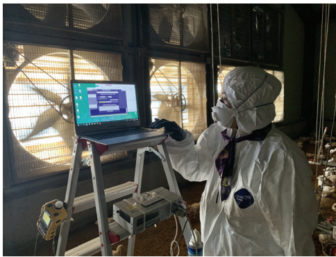
(c) Sampling set installed in front of tunnel-exhaust fans
