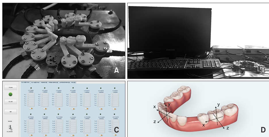
Figure 1. The force measurement system. A , Three-dimensional-printed resin teeth connected separately with the multi-axis force/moment transducer by hexagonal screws. B , The computer linked with the measurement system. C , The real-time visualization window of Angelalign Mechanical Measurement Software (Wuxi Angel Align Biotechnology Co., Ltd., Wuxi, China). D , The coordinate system for the forces and moments measured. The y-axis runs through the center of tooth and parallel to the long axis of this tooth. The x-axis is oriented parallel to the mesiodistal direction of teeth. The z-axis represents the labiolingual/buccolingual force.
