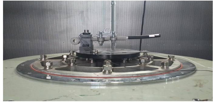
Fig. 10. Test setup for step stress testing
