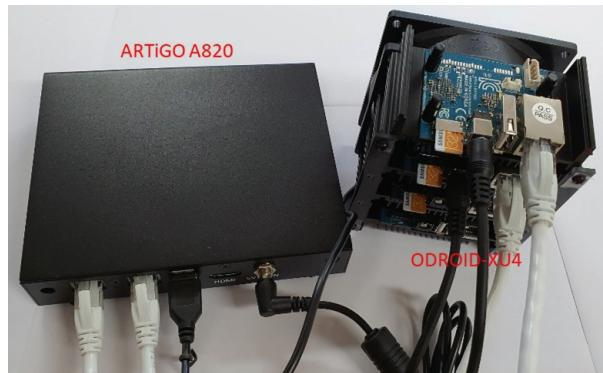
**Fig. 10.** ODROID-XU4 and ARTiGO A820 for remote execution code simulation.
