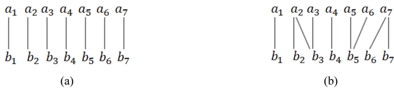
Fig. 2. Example of computing the DTW distance: (a) Euclidean matching and (b) DTW matching.
