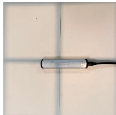
Fig. 2. Air kerma measured on X-ray table without phantom
