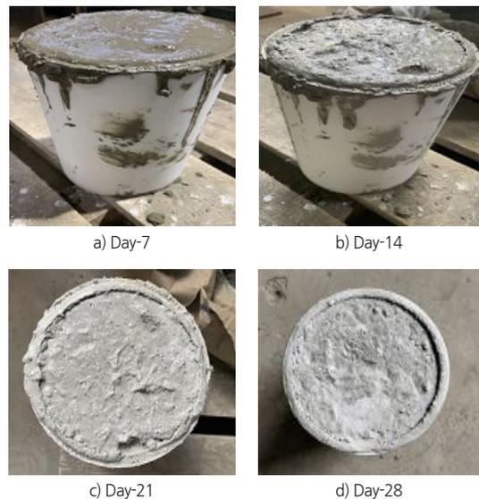
Fig. 7. Filament formwork curing
