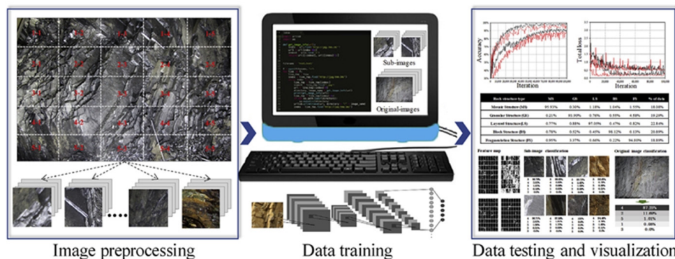
Fig. 5. Classification process of tunnel faces using Inception-ResNet-v2 model (Chen et al., 2021)
