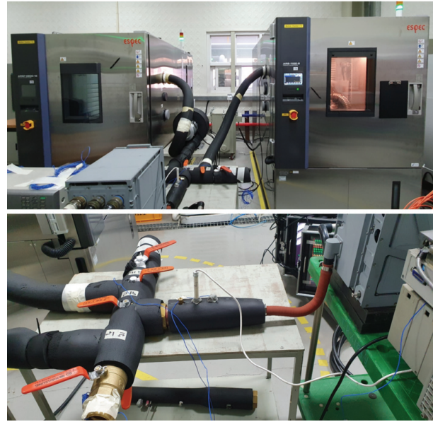
Fig. 11. Configuration of rapid temperature change test equipment
