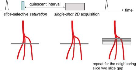
Fig. 6. Principle of quiescent interval single-shot imaging (QISS). The pulse sequence consists of thin saturation preparation, quiescent interval period, and single-shot 2D acquisition. During the quiescent interval, saturated static tissues recover only partially while fresh upstream arterial blood flows into the imaging volume. This is repeated multiple times for neighboring slices without a slice gap to form 3D volume of angiogram.
