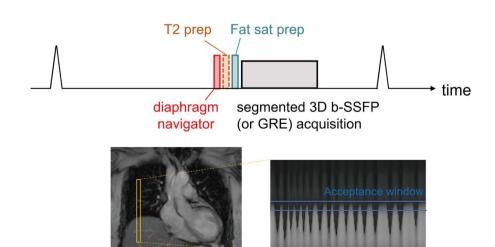
Fig. 7. Principle of free-breathing 3D coronary angiography. The pulse sequence is cardiac gated. It applies respiratory navigator, T2 preparation, fat saturation, and segmented 3D acquisition. The respiratory navigator applies pencil beam-shaped excitation across the liver-air interface to obtain 1D signals over cardiac cycles. It decides whether to record or abandon data segments obtained in the same cardiac cycle based on a pre-defined acceptance window.
