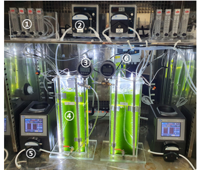
Fig. 3. Continuous MMBR reactor set-up (① Flow meter, ② Inlet pump, ③ Pressure gauge, ④ MMBR, ⑤ Outlet pump, ⑥ pH controller).
