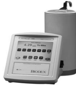
Fig. 3. When using the dose calibrator, the radioactivity source was set to a volume of 0.1 ml in a 1 cc type syringe, placed in a dedicated sample holder, and then radioactivity was measured.
