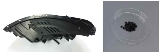
Fig. 6 Sample of Housing & PP pellet
