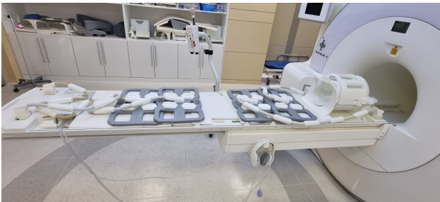
Fig. 2. Attenuation correctable torso imaging matrix coil for PET scan
