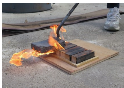
Fig. 2. Treating Nakdong-iron on the surface of paulownia wood.
