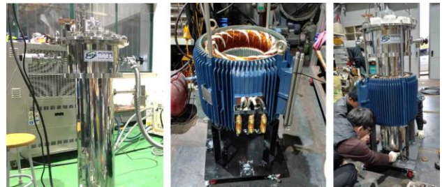
Fig. 4. Photographs of assembly cryostat part into induction motor.
