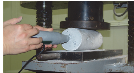
Photo 2 Schmidt hammer test
