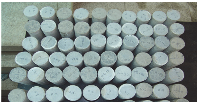
Photo 1 Curing of test specimens
