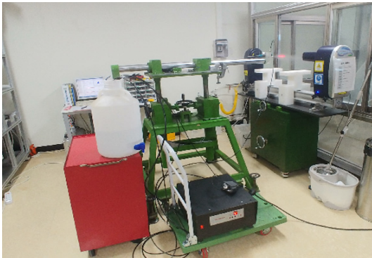
Fig. 2. Experimental setup to measure the FOG droplet diameter
