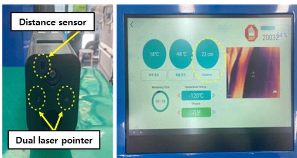
Fig. 4. Photo of Nitrogen Injection Gun to Improve the Accuracy of the Distance Measuring Sensor and GUI Screen Display.
