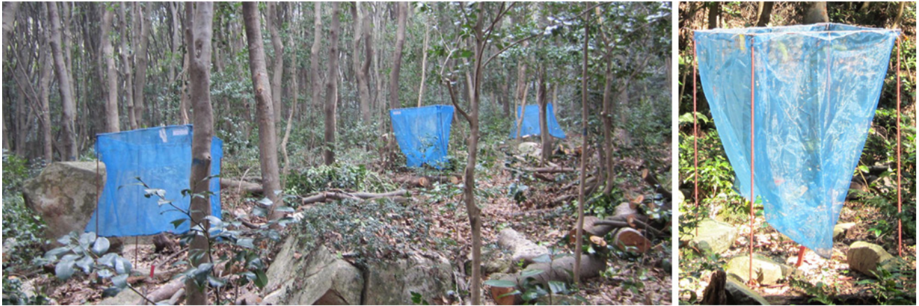
Figure 3. Seed trap with one meter by one by one point five high.
