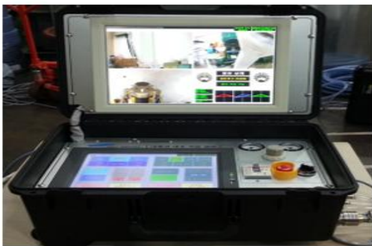
Fig. 14 Robot controller layout
