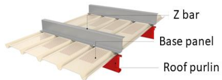
Fig. 2 Internal structure of metal panel roof
