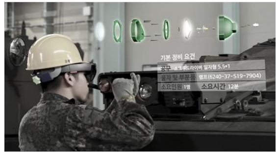
Fig. 7 AR-based maintenance manual visualization
