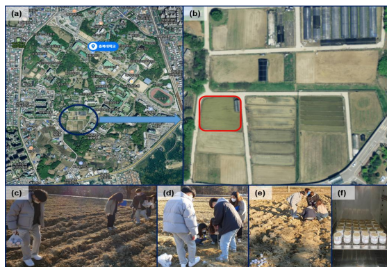
Fig. 1 Paddy Fields for obtaining data such as pH, Electrical Conductivity (EC), moisture content, Cone Index (CI) and soil classification; (a) map of the site where paddy field is located; (b) paddy field where soil is taken in Chungbuk National University; (c) soil compaction by men; (d) measuring CI; (e) obtaining soil samples at 30 points; (f) drying moisture of the sampled soil in the oven
