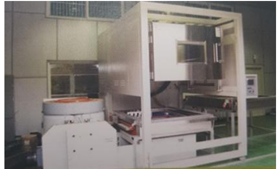
Fig. 2 Long stroke vibration test equipment
