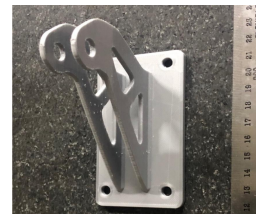
(c) FDM 3D printed door hinge with remove support Fig. 2 FDM 3D printing process of door hinge parts
