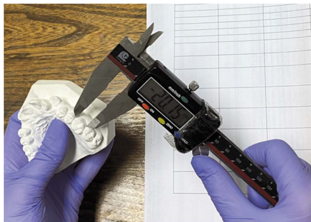
Fig. 1. Making a measurement on a plaster cast using a digital caliper.
