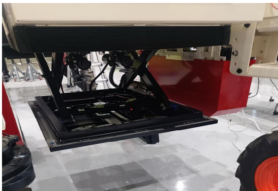
Fig. 1 Assembling Auto Module Changer with Farm bot
