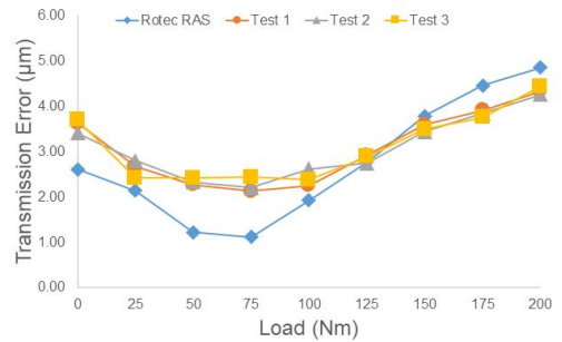
Fig. 12 Result of counterclockwise transmission error test
