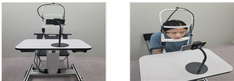
FIGURE 8. The device for the pupillary light reflex measurement
