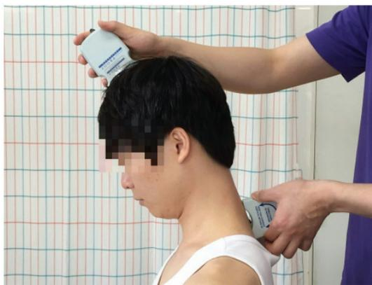
Fig. 1. Digital dual inclinometer (HOGGAN PROOF Preferred, HOGGAN HEALTH, USA, 2006).
