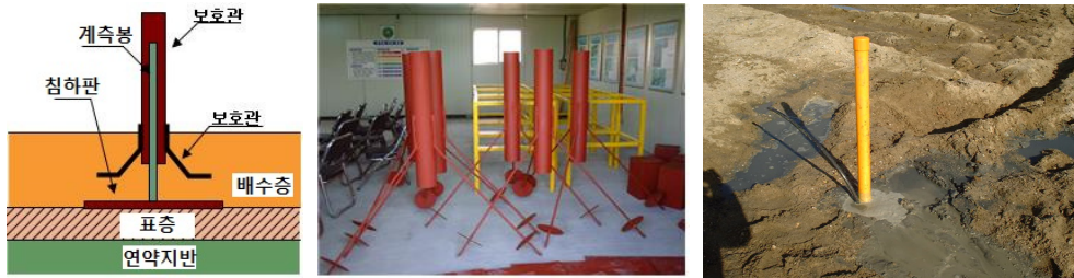
Fig. 1. Ground settlement plate installation concept and installation
