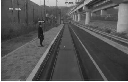
Fig. 10. TTC, Predicted Collision Point & Warning Message
