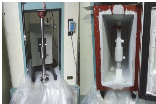
Fig. 1 Photograph of experimental apparatus for compression test at room and cryogenic temperature
