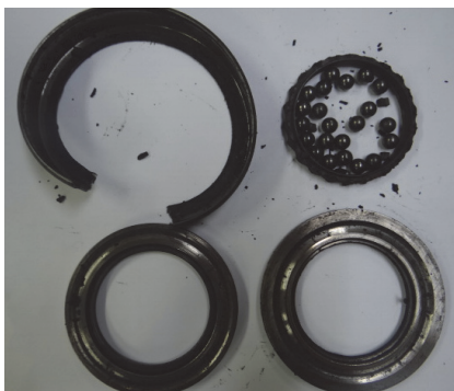
Fig. 5 Disassemble failure bearing
