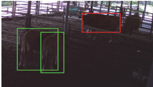
Fig. 6 Objects detected simultaneously in visible light and thermal image are displayed in green
