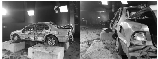
Fig. 11 Vehicle damage due to explosion of hydrogen tank
