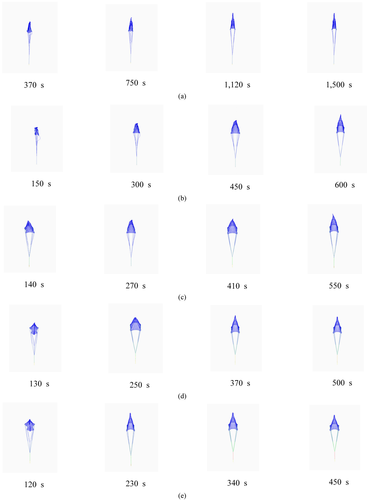
Fig. 8. Shape of offshore stow net during opening process at 25%, 50%, 75%, 100% ((a) 0.5 knot, (b) 1.0 knot, (c) 1.5 knot, (d) 2.0 knot, (e) 2.5 knot).
