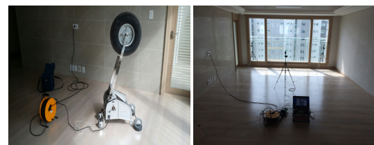
Fig. 2. (Color available online) Measurement for heavy-weight impact floor noise (Bang machine and receiving room).
