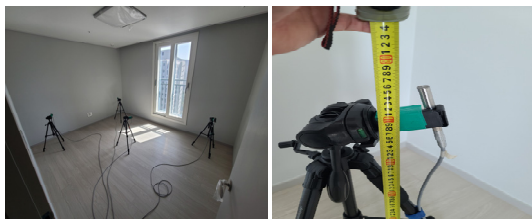
Fig. 1. (Color available online) Measurement detail and microphone position for elevator noise.
