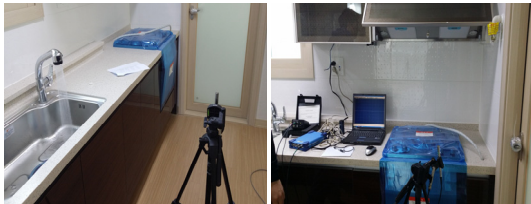
Fig. 3. (Color available online) Measurement site and details for sink water supply noise and fume hood operation sound.
