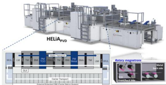
**Fig. 12.** HELiA PVD system with rotary magnetron sputters (Meyer Burger Corp.)
