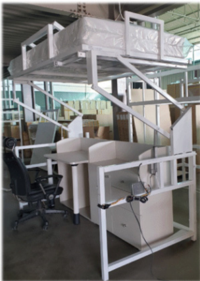
Fig. 12 Prototype of height adjustable bed using linear actuator
