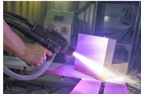
Figure 2. Arc thermal metal spraying method
