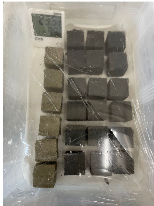
Fig. 2. Wet curing of specimens
